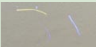
protective fibres blue and yellow fluoresce
