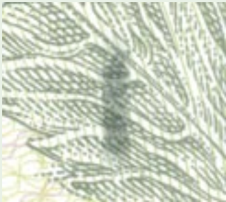
no effect on protective strip when Pole Tester is applied
